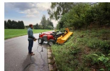
is the first radio-controlled equipment carrier with a true hybrid drive. The vehicle concept is based on a Kubota petrol engine with 48 HP, a generator flanged directly to the flywheel, 4 electric wheel motors, and a battery pack. The Metron
