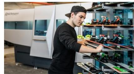
The filled wagon can be docked directly at the machines, eliminating the need for time-consuming reloading. After docking, the automatic service unit takes care of all the work steps automatically, including picking up the skis in pairs in the automatic units and depositing them back in the transport trolley. Your service personnel can take care of other important tasks in the meantime.
