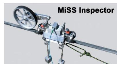
Magneto-inductive cable tester for accredited testing institutes as well as cable and cableway manufacturers. Wireless data transmission with Wi-Fi and the ability to test cables remotely via the internet are factors which make the MiSS
